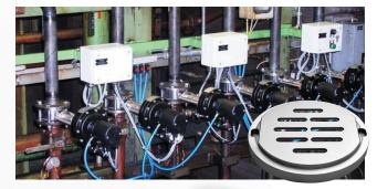
Sliding gate valves controlling the flow in an aluminium rolling plant: the aggressive and abrasive rolling emulsion is no problem for these valves which provide ultimate functional reliability by their two slotted plates sealing against each other. High-level leak-tightness despite suspended particles and a long service life create optimal conditions for economical production.
